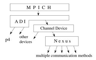
Figure 2: The Nexus implementation of MPI is constructed by defining a Nexus instantiation of the MPICH abstract device interface. In the first version of MPICH/Nexus, this was achieved via an intermediate channel device, as shown here; more recently, a tighter integration of MPICH and Nexus has been achieved by providing a full Nexus implementation of ADI-2.
