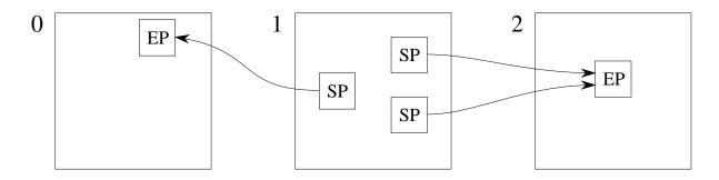
Figure 1: The communication link and its role in communication. The figure shows three address spaces; three startpoints in address space 1 reference endpoint in address space 0 and 2.
