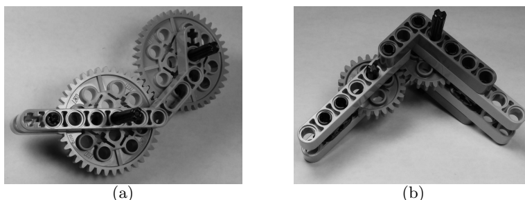
Fig. 3. (a) The exact Pythagorean triple 3-4-5 with the hypotenuse formed solely by gears. (b) the approximate Pythagorean triple 1-3-3 that has the greatest absolute error (0.16) that seems workable in practice.
