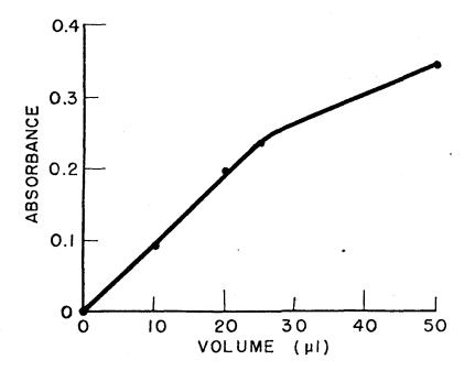
Figure 1: Curve obtained using pipettors of various volumes. A standard aluminum sulfate solution, 100 ug of Al per liter, was used.
