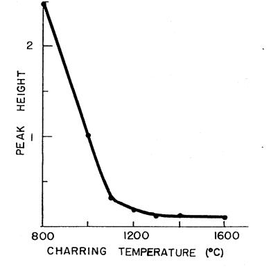
Figure 4: Minimum charring temperature for serum and urine.
