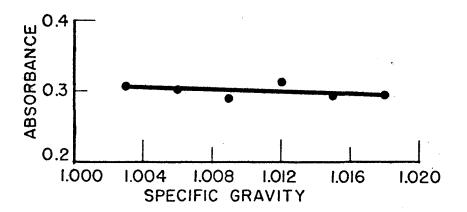
Figure 12: Graph demonstrating the effect of specific gravity on urinary aluminum determinations. Specific gravity determined from refractive index.
