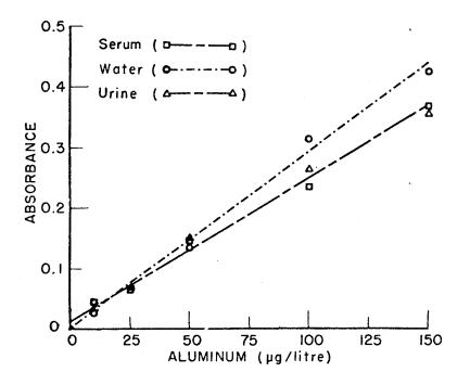
Figure 8: Standard curves showing the effects of different matrices.
