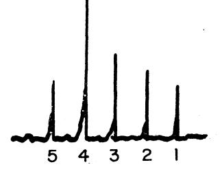
Figure 2: Chart recorder tracing demonstrating the need for removal of the residue from the graphite tube between analyses of serum and plasma. During five consecutive analyses of a sample, the residue was not removed until after the fourth determination. This was especially necessary if drying was at 100 °C.
