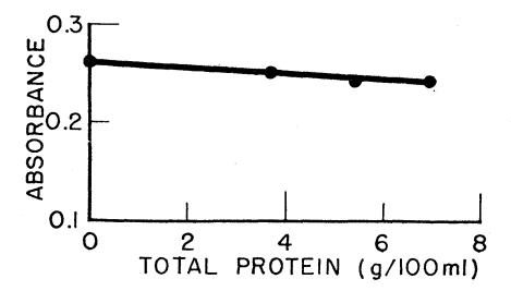
Figure II: Graph demonstrating the effect of protein content on serum aluminum determinations. Total protein determined by the Biuret method.
