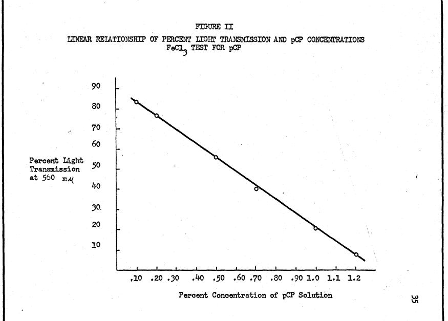
confines of this criteria. This made it possible that any test solution containing an unknown concentration of pCP could be evaluated as to its percent light transmission and its concentration determined by comparison of these values to the standard. (Table 5, Figure III)
