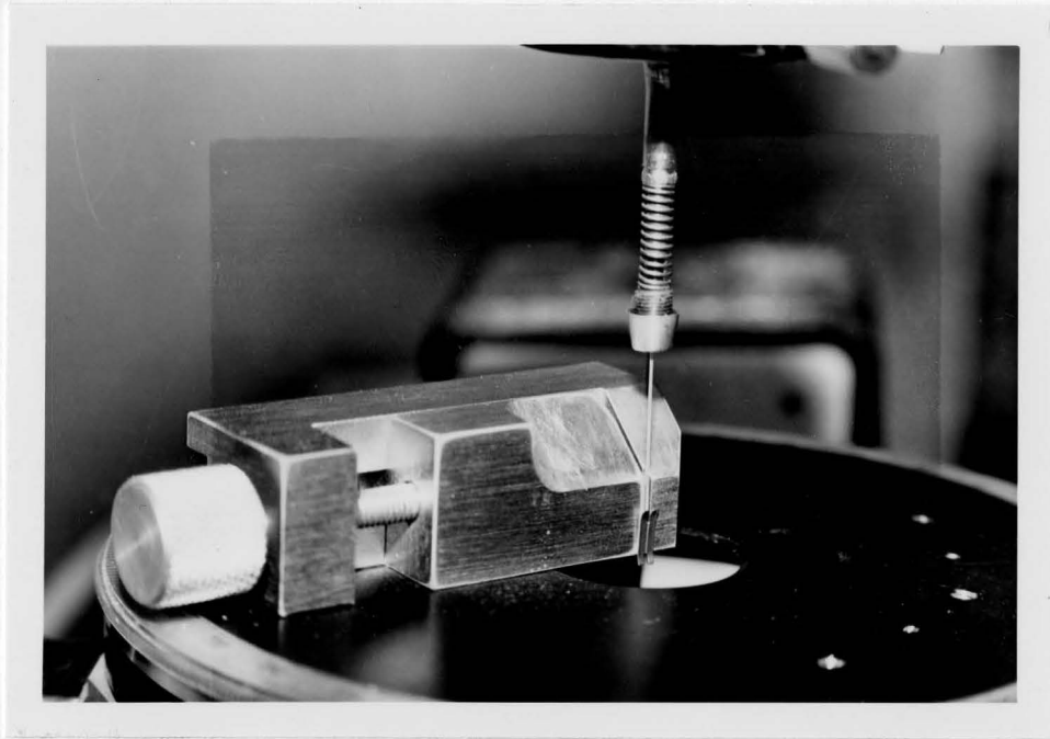
Figure 2. Holding Vise Mounted to the Rotatable Stage
