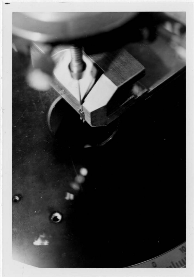
Figure 5. Upper view of tube holding vise mounted on the stage.
