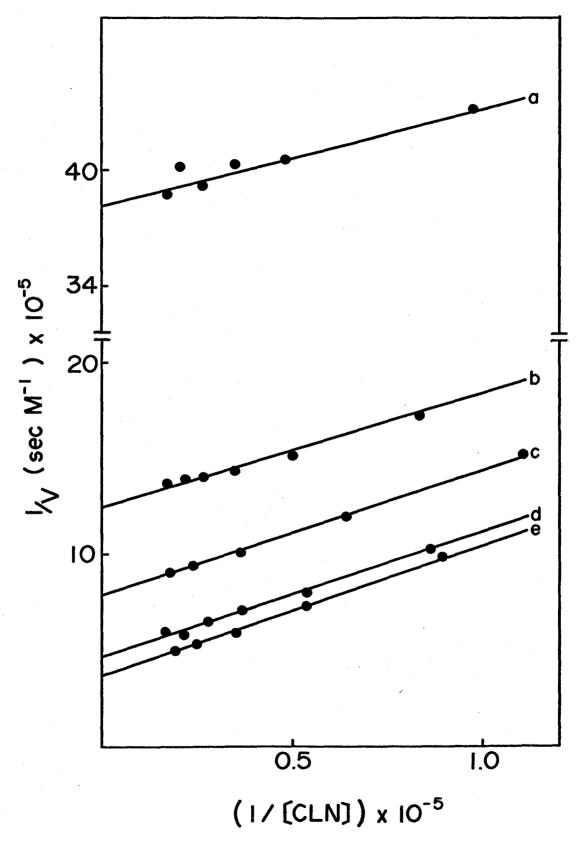
different concentrations of gly-gly. A series of essentially parallel lines are obtained with V increasing with increasing nucleophile concentration.
