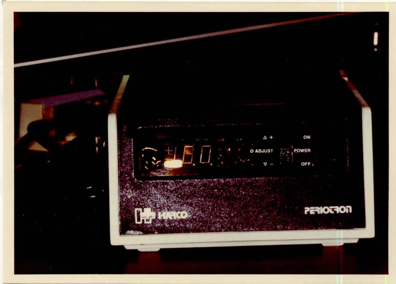
Figure 1. Periotron (Clinical GCF Meter - Harco Electronics LTD, Winnipeg, Canada.)
