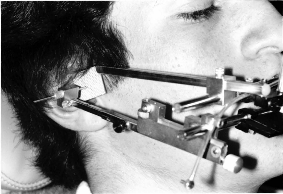
Figure 4. Hinge axis location of the posterior reference points on subject using the Denar Hinge Axis Locator.
