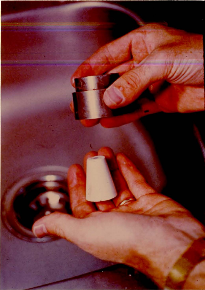
Figure 11. Plaster mold released from flask before separating the plaster and the hard stone from the ceramic coping.
