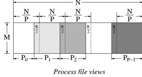
Figure 7: The process file views for the column-wise overlapping I/O using process rank ordering approach. With the overlapping access removed, all  $P$  I/O requests can be performed simultaneously while MPI atomicity is guaranteed.
