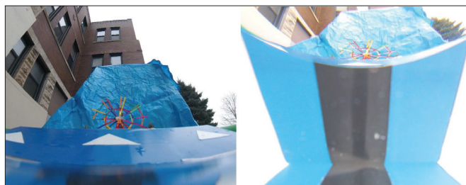
Fig. 3. This figure shows the difference between what a racer sees in the game and what the racer should see if physics is properly applied. We take the image on a ramp, with the left image showing an image taken with no water present and similar to what the player would see in the actual game. The right image shows an image taken from the ramp from the same position, but with water placed such that the camera is below the water line. Notice that the effects of Snell's law and total internal reflection are apparent in the right image and is indicative of what the player should see.
