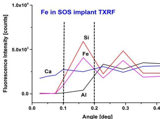
Figure 3: Fluorescence Intensity as counts in dependency of incident X-ray beam angle for a  $5 \times 10^{14}$  atoms/cm<sup>2</sup> Fe implant. Implanted depth at  $395 \pm 130 \text{ \AA}$  (Kitts *et al.*,2009a,b).
