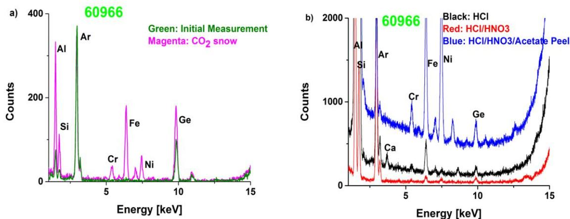
Figure 1: TXRF spectra a) collected with PicoTax after routine UPW/O<sub>3</sub> cleaning (green) and after CO<sub>2</sub> snow cleaning (magenta) and b) collected with S2PicoFox after HCl/H<sub>2</sub>O<sub>2</sub> (black), HNO<sub>3</sub> (red) and acetate peel (blue) treatment.
