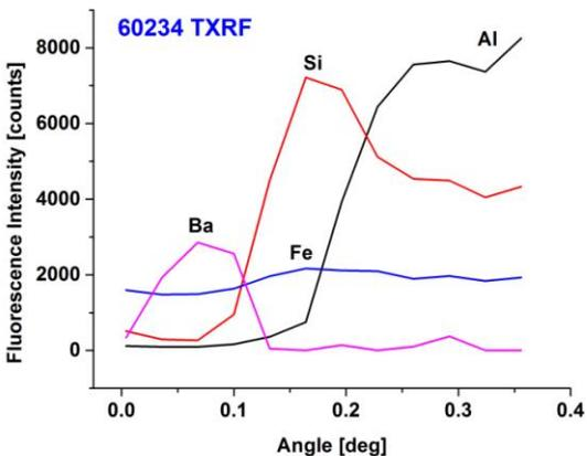
Figure 4: Fluorescence Intensity versus incident beam angle recorded with bench top TXRF for Genesis flight sample 603234.
