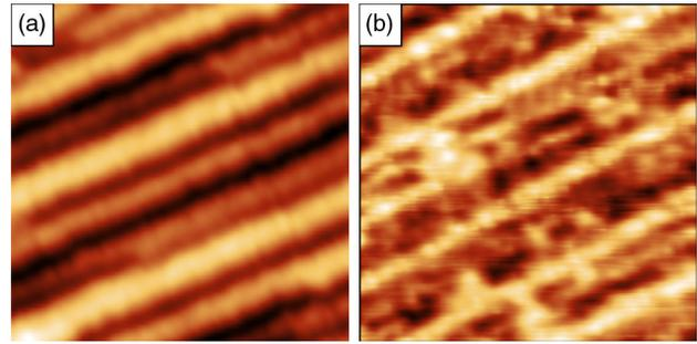
FIG. 3. (a) STM image of the clean Pt(553) surface.  $V = 1$  V,  $I = 200$  pA,  $T_{STM} = 25$  K,  $8 \times 8$  nm<sup>2</sup>. (b) STM image of the water-covered surface.  $V = -0.90$  V,  $I = -9$  pA,  $T_{STM} = 25$  K,  $8 \times 8$  nm<sup>2</sup>.
