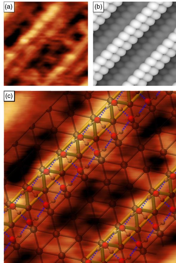
FIG. 4. (a) STM image of  $D_2O$ -covered step edges on Pt(553).  $V = -1$  V,  $I = -9$  pA,  $T_{STM} = 25$  K,  $4.5$  nm  $\times$   $4.5$  nm. (b) STM simulation of water adsorbed on Pt(553), bright areas are oxygen atoms of water, darker areas are located at Pt terraces,  $V = -0.9$  V. (c) Overlay of atomic positions of DFT and STM imaging,  $V = -1$  V,  $I = -9$  pA,  $T_{STM} = 25$  K,  $4.5 \times 4.5$  nm<sup>2</sup>.
