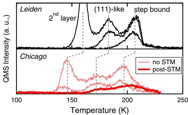
FIG. 2. TPD spectra of water desorbing from Pt(553).
