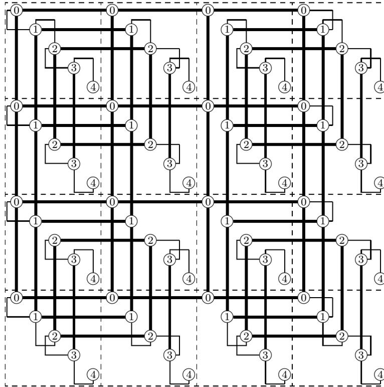
Figure 5-2: The  $4 \times 4$  tree of meshes  $T_{2,4}$  laid out by the fold-and-squash method. Each node is labeled with its level in the underlying tree. The “cubies” are outlined with dashed lines. Mesh edges are shown with thick lines and are routed between cubies. Tree edges are shown with thin lines and are routed within cubies.
