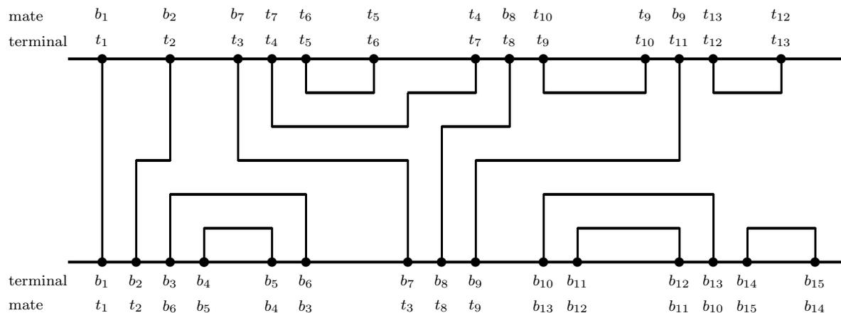
Figure 7-1: A representative single-layer channel routing problem. Each terminal  $T$  among the top terminals  $\{t_i\}$  or the bottom terminals  $\{b_i\}$  must connect to exactly one terminal  $mate(T)$ .
