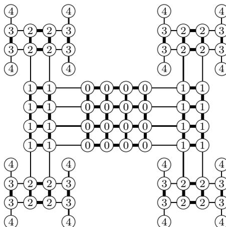
Figure 5-1: The  $4 \times 4$  tree of meshes  $T_{2,4}$  in the H-tree layout style. Each node is labeled with its level in the underlying tree. The “mesh” connections are shown with thick lines, and the “tree” connections are shown with thin lines.
