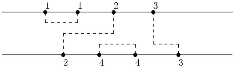
Figure 1: An example of single-layer channel routing
