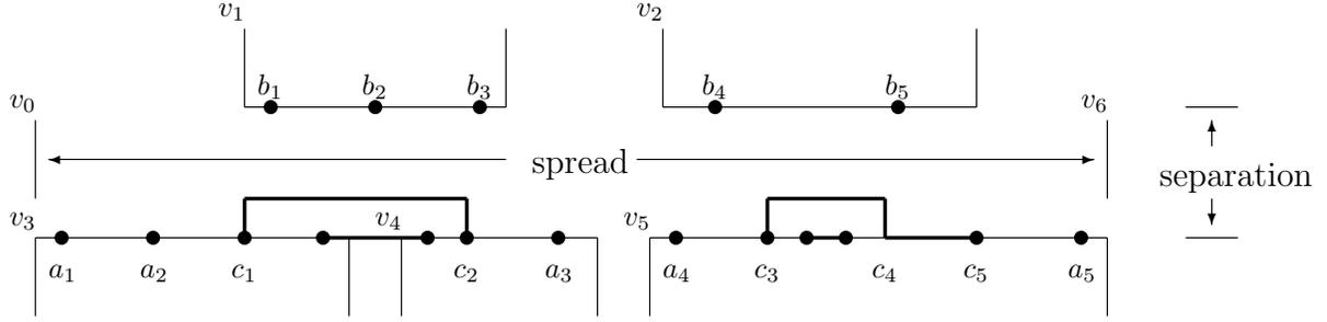
Figure 3: Two sets of chunks on either side of a channel. Variables are assigned to the horizontal position of each chunk's left edge.
