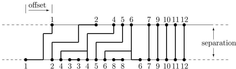
Figure 1: A single-layer channel and a routing that achieves the minimum separation. The number above or below each terminal identifies the net to which it belongs.
