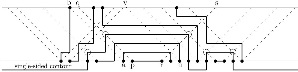
Figure 2: Only those  $45^\circ$  cuts from bottom terminals shown with dashed lines need be checked. The hollow circles mark the convex corners of the contour of single-sided nets.
