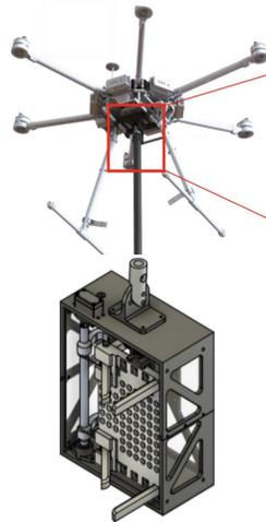
Figure 1. Illustration of the drone and deployment/retrieval system.
