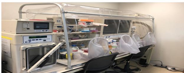
Figure 2. Anaerobic Hood Chamber
