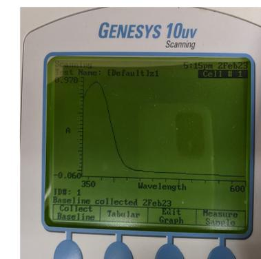
**Image 3. Example of Scan on the Genesys 10UV Spectrophotometer**
