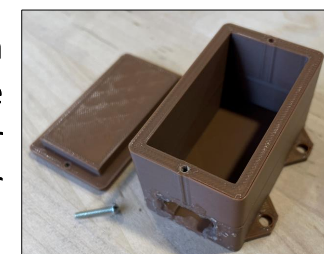
Figure 6: 3-D Printed Protective Housing for ESP32W Microcontroller showing latches for fastening, lid, and screw
