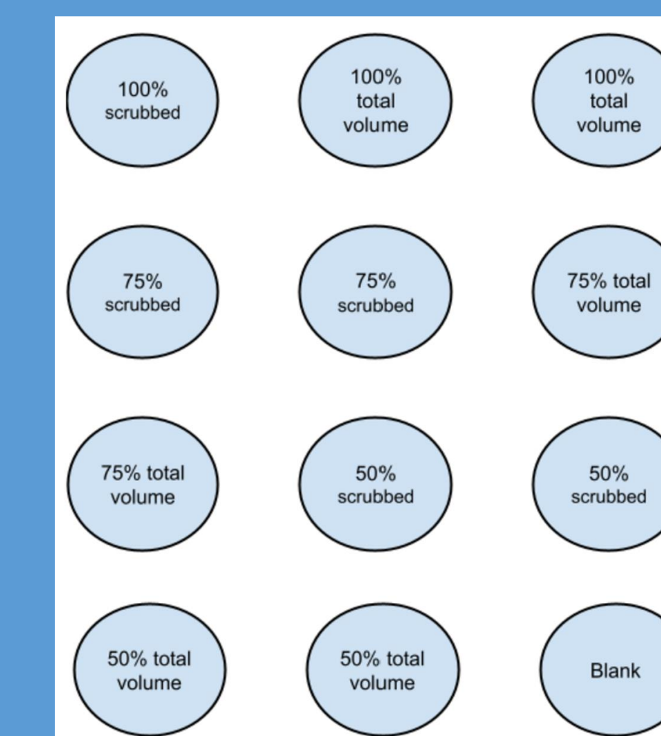
Figure 3. Reactors schematic. Demonstrates how the reactors are organized and filled.
