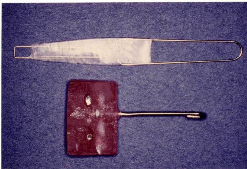
Figure 2. Special loading jig and the hook, which would be mounted on the upper part of Instron machine.
