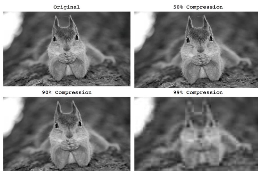
Figure 4. PCA Compression Examples. The original image is tiled as 32x32 pixel blocks - 15 along the width and 10 along the height. The original image (0% compression) uses all 1024 PCA components for each image patch. The 50% compressed image uses the first 512 PCA components, and is essentially indistinguishable to the naked eye. 90% compression uses only the best 100 components reducing the file size to 10% of the original. Note, that even when the image patches are represented using only 10 PCA components (1% of the original file size), the image is still recognizable (Hofman, n.d.).
