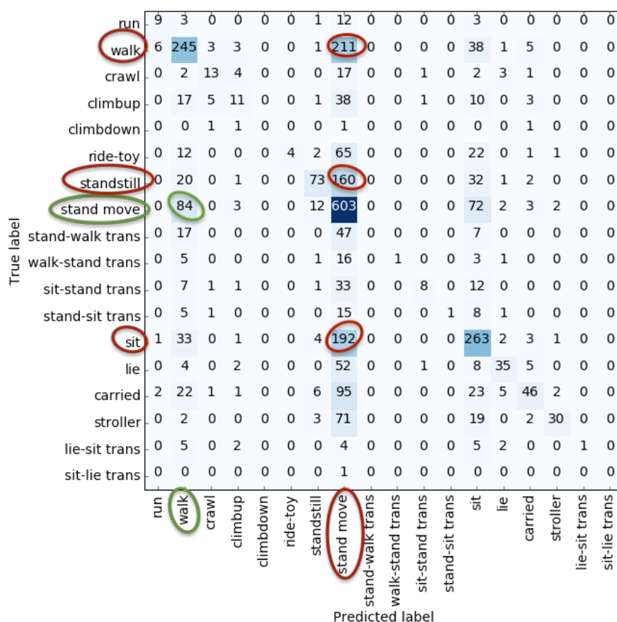
FIGURE 10: Confusion matrix derived from random forest classifier highlighting how "stand move" is misclassified
