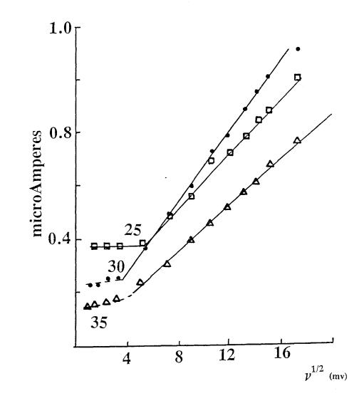
Fig. 7 Maximum current obtained as a function of the scan rate for SAz-1 spin-coated Pt electrodes in 2 M NaCl.
