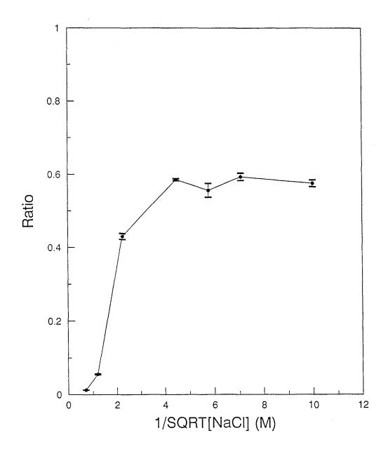
Fig. 11 A plot of ratio  $(i_{pcme}/i_{bare})$  vs. 1/SQRT[NaCl] obtained for 4 mM Na<sub>4</sub>[Fe(CN)<sub>6</sub>] probe at 1  $\mu$ l 35 g/l SWy-1 SPCME.
