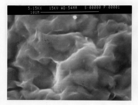
Fig. 4. SEM image of 1  $\mu$ I SWy-1 spin-coated film viewing from the back side of the film.
