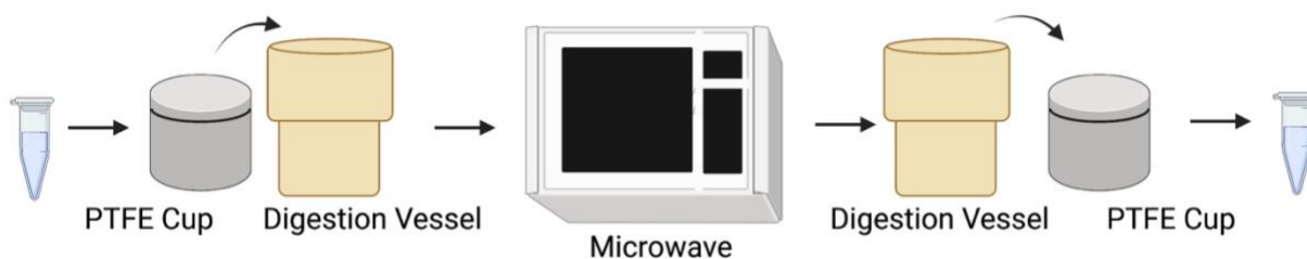
Figure 12. Schematic representation of microwave-assisted acid digestion
