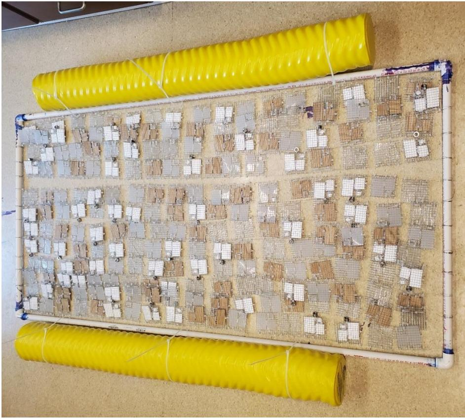
Figure 3. Assembled raft showing randomized placements of substrates, the PVC pipe frame, and yellow floats. Scale: the PVC frame is 152.4 x 76.2 cm.
