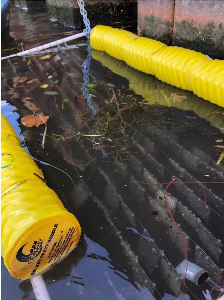
Figure 4. Deployed raft showing substrates submerged near the water surface, attached to the seawall. The HOBO data logger is in the foreground.
