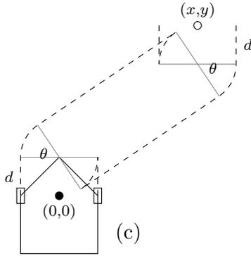
Figure 3: Here we use rotations but with straight segments of distance  $d$  at the beginning and end of the path so the rotations can occur without banging into horizontal boundaries abutting the robot's beginning and ending positions. The distance  $d$  in this picture is exaggerated for visual effect.
