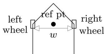
Figure 0: We will sketch our robot as shown, with a pointed front and a reference point centered between the two independently-driven wheels; there is also an assumed third balance point, for example a caster wheel in the back.
