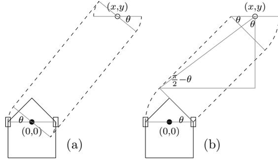
Figure 2: The paths of the robot wheels under general navigation, using rotations in (a) and swings in (b).
