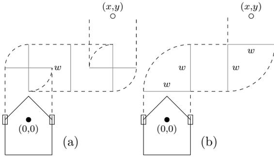
Figure 1: The paths of the robot wheels with horizontal and vertical navigation, using rotations in (a) and swings in (b).
