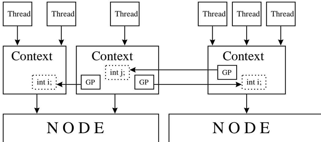
Figure 1. Nodes, Contexts, Threads, and Global Pointers
