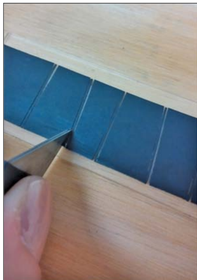
Fig. 3. A double-slit pattern is cut into black electrical tape adhered to a microscope slide using two razor blades taped together.
